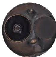
Cylinder head before P.i. treatment.
