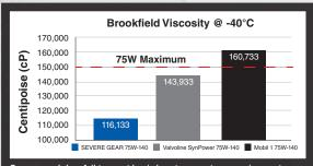
Some gear lubes fail to meet basic low-temperature requirements.
