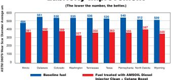
The ASTM D975 diesel fuel standard specifies a wear scar below 520  $\mu m$  in ASTM D6079 testing, while the Engine Manufacturers Association (EMA) specifies a wear scar below 460  $\mu m$ . Testing reveals AMSOIL Diesel Injector Clean + Cetane Boost provides significant lubricity improvement in diesel fuels found across the U.S., delivering improved wear protection.
