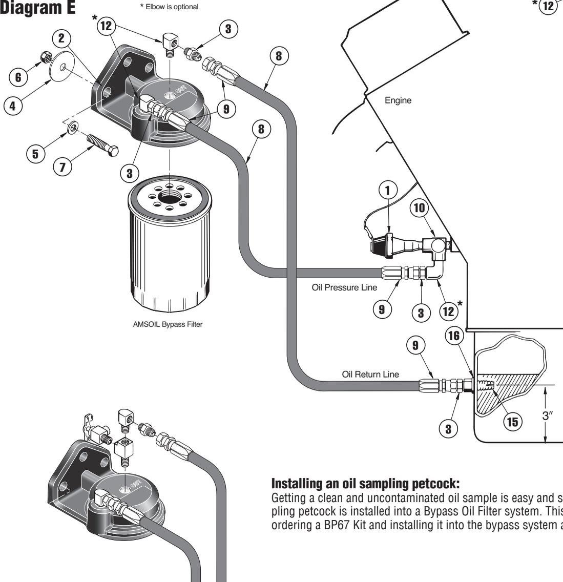
**Note:** When installing self-tapping hollow bolt to oil pan, locate approximately 3" from bottom of sump. Avoid installing on or near any unusual pan formations which might indicate an internal obstruction.
