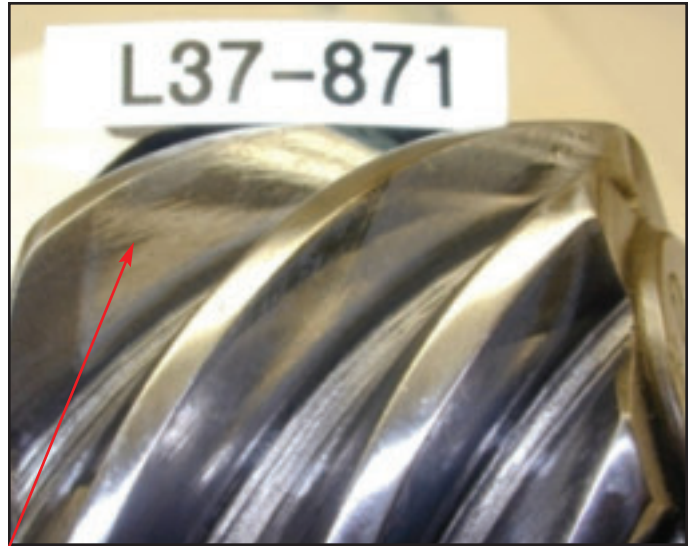
Pinion gear - original machine marks still present.
