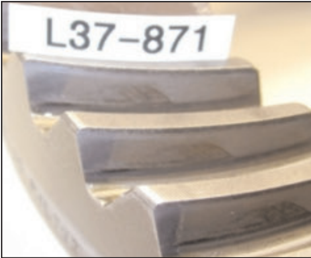
Ring gear exhibits very low wear.
